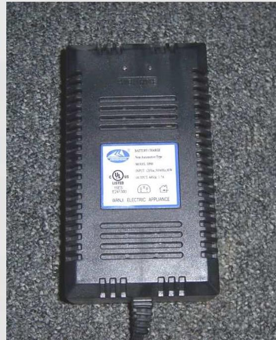
Replaced with a linear (non-switching) power supply
