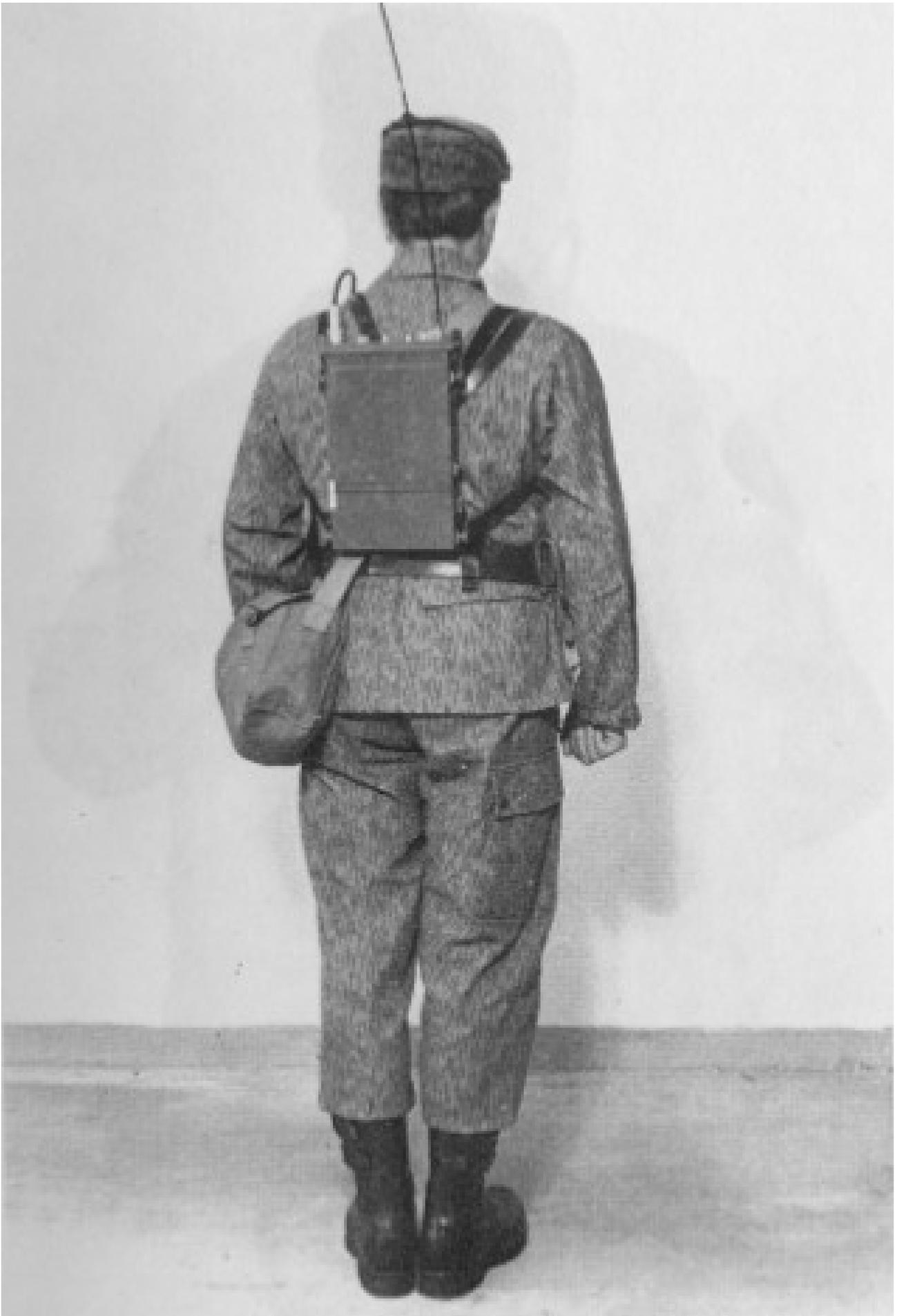
*Figure 7: Radio worn on the back – rear view*
