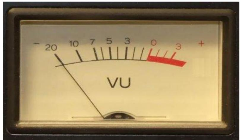
**Audio level meters should adhere to the official VU standard for response to signals, but don't always, even if they are marked 'VU' on the face.**
